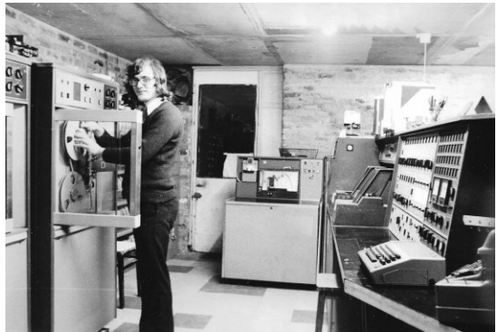
Galdor's Andy Keene loads a half inch magnetic tape. The keyboard is a Galdor addition
