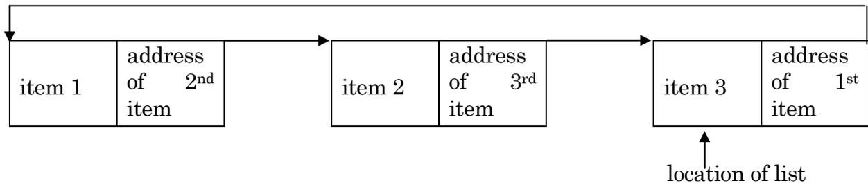
An empty list is represented by the address 0. All the preloaded auxiliary statements for manipulating circular lists assume these conventions. Initially all the register pairs in the area of store allocated for circular lists are linked together and the address of the first is in  $\beta_{89}$ . Words are removed from and returned to this main chain as required by the appropriate adjustment of links and the  $\beta_{89}$  register.
