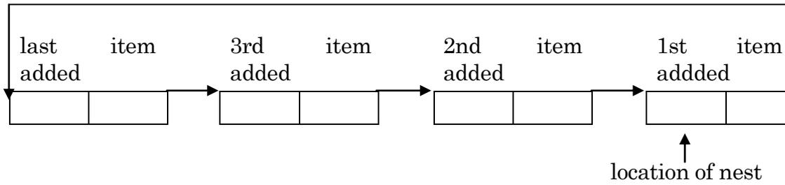
Thus items in a list are most easily processed or removed from the first through the last, whilst in the case of a nest this order is reversed. In other words, a nest is a last-in first-out device sometimes referred to as a pushdown list.
