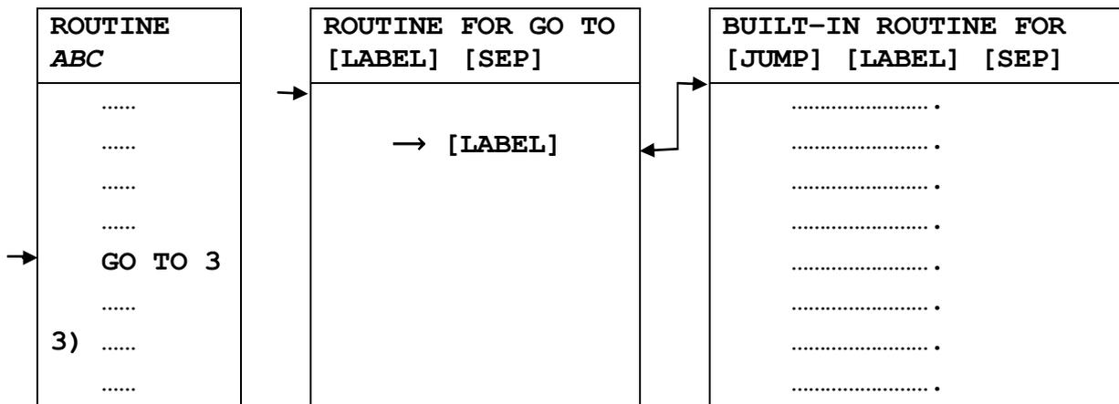
When this instruction is reached control is transferred to the GO TO [LABEL] routine as shown, which at the → [LABEL] instruction further transfers control down to the built-in routine for [JUMP] [LABEL], which has finally to transfer control back to label 3 in the routine ABC. Thus the analysis record of [LABEL] which is carried forward in the process must contain the label number 3 and a reference to the routine ABC.
